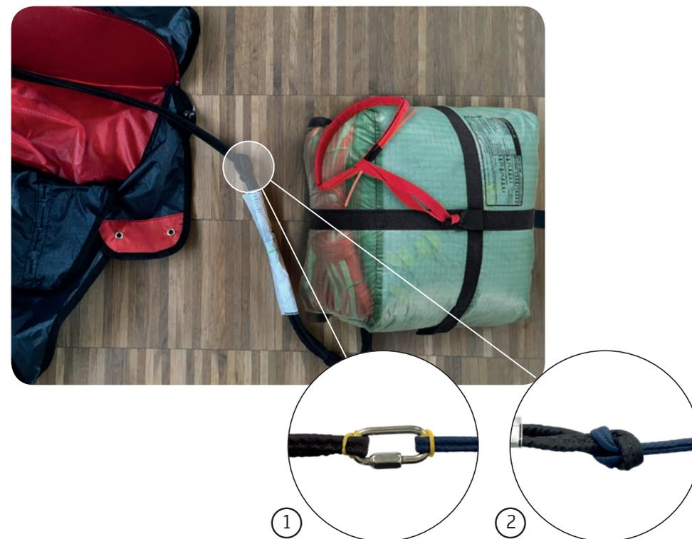
It is important to ensure that the connection is centered, that is, the two connecting lines leading to the shoulder straps are of the same length. If the harness does not have an integrated attachment possibility for the reserve chute on the shoulder straps, then the reserve chute connecting line can also be attached to both main carabiners.
