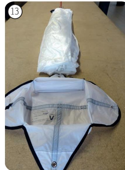
**13.** Now fold the reserve chute with a „double-S fold“ (see graphic) and place the reserve container with the line pocket in the direction of the base/main riser.
