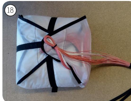
**18.** Secure the fourth and final rescue flap with the remaining line length from step 16.
