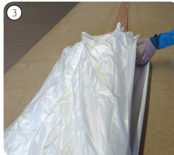
3. The SALSA is a cruciform rescue parachute with four corner points, so lay out the canopy with one corner at the bottom, one on the left, one on the right and one on top. Start with the first corner at the bottom and smooth the material by running your hand along it on the table.
