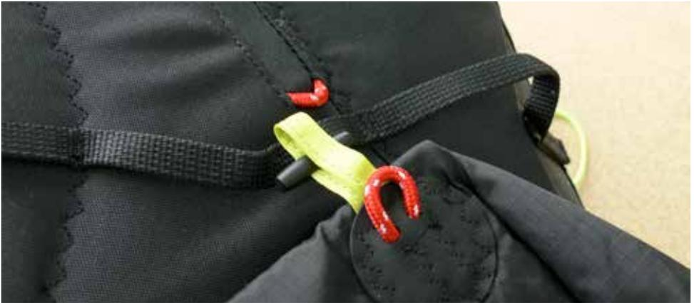
To begin, the toggle of the preferred side (left or right) is led through the corresponding red loop of the leg strap (left to left, right to right).
