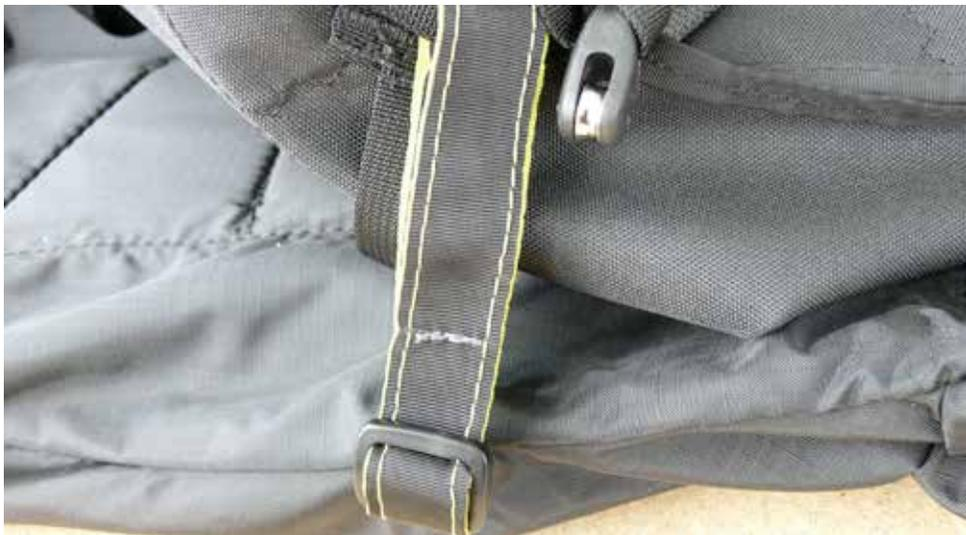
On the side, at the height of the speed bar pulleys, there is a strap on both sides for connecting the airbag. Also for this purpose, there is a strap and buckle on the airbag. Feed the strap through the loop. Next, the strap is pulled through the buckle on the airbag and then looped back through. This procedure should be performed left as well as right in the desired sequence.
