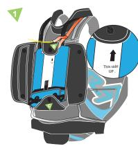
1. Position the pod while respecting the correct direction ( see marking «this side up») as well as avoiding any connection bridle twist. Fold the upper and lower flaps.
