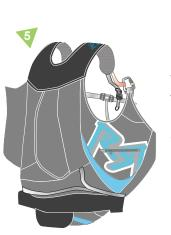
5. Fold over the shoulder flap then the riser cover flap for the under-seat parachute location.
