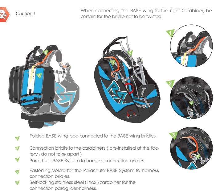
1. Position the pod correctly (logo "This side up" with the arrow pointing upward). Pull the the connection bridle out of the pod and place it over the BASE wing connection risers. Be certain not to have any twist and for the bridle not to be wrapped around the risers.
