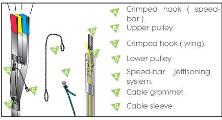
1. Remove the crimped hook and pull out the speed-bar line from the pulleys. Tuck away this line with a piece of Velcro or tape to prevent any interference with the system.
