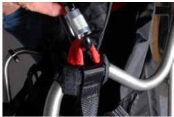
Fasten securely using the Velcros®, then push the glider's self-locking carabiner through to connect the wing's risers.
