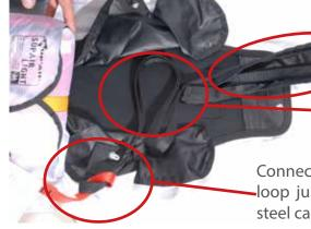
Position the risers inside the bottom section of the pocket with a bit of slack to adjust them at the end of the installation.
