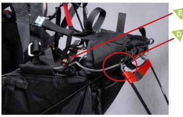
Push the accelerator cord and the elasticated line through ring ""D"".
