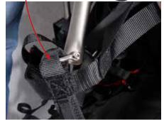
Fasten the bars ends to the harness loop straps using a shackle.
