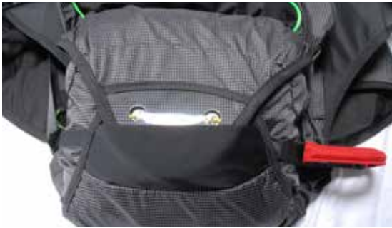
The yellow cable locks the reserve parachute pocket flaps in place. Tuck the upper flap inside its lower stretchable pocket. Check before every flight for the yellow cable to be properly inserted through the two loops keeping the reserve parachute pocket securely
