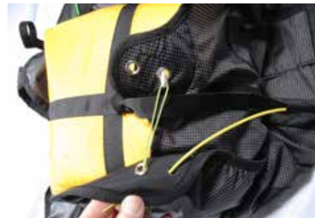
Push the loop through the lower flap grommet. The yellow cable will also be pushed through the lower flap guide located near the grommet.
