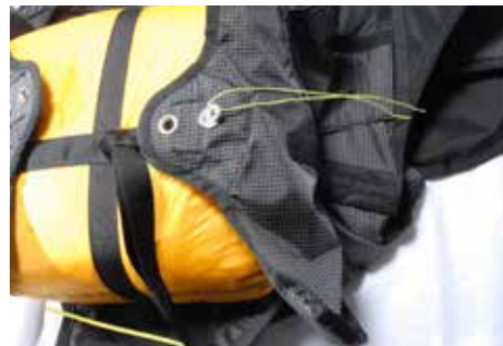
Push the cord through the right loop ( if the handle is located to the right ).
