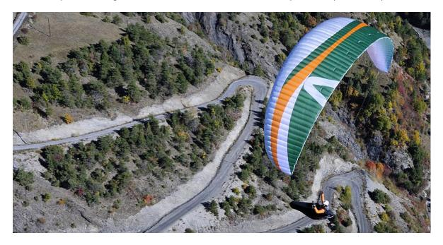
The POISON3 has a phenomenal attraction to thermals: there is hardly another glider that bites into thermals like this one, although the canopy shoots forwards somewhat. For this reason, flying into strong thermals requires an adept hand, which can absolutely be classified as a positive characteristic. The POISON3 has a natural tendency to fly flat curves, still possible while climbing steeply, without a tendency to spin. To turn
